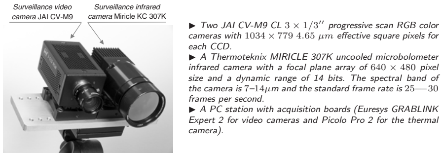
Fig. 4. A setup of a pair of video and infrared cameras for surveillance
